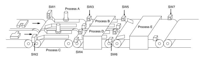
The following diagram demonstrates the flow of processing and the switches that are used for execution control. Here, process A and process C are started together. When process A finishes, process B starts; when process C finishes, process D starts. When both processes B and D have finished, process E starts.
